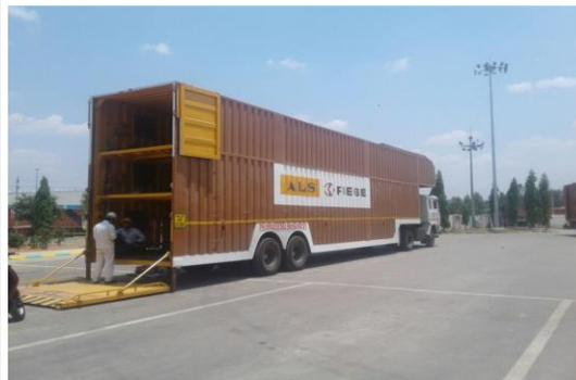
Trailers of capacity 120 vehicles are used for dispatch of two wheelers from HMSI
